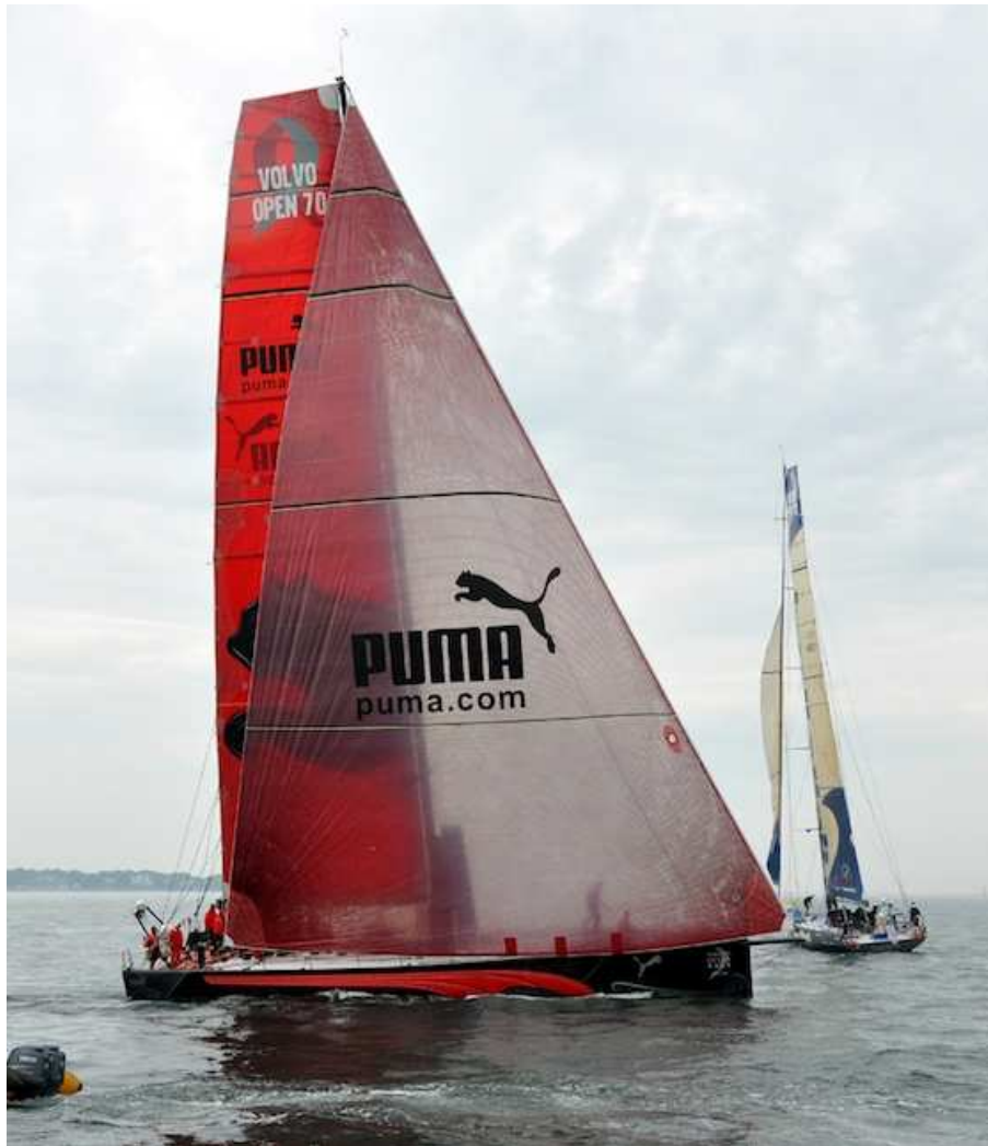
Puma, upwind before racing with its giant light-air headsail. Photo by Bill Bolin
